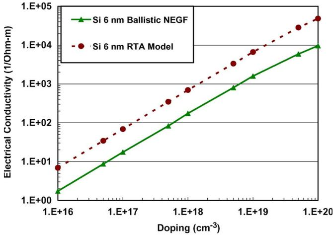
Fig. 4. Electrical conductivity versus doping for silicon films using the NEGF and RTA models.
