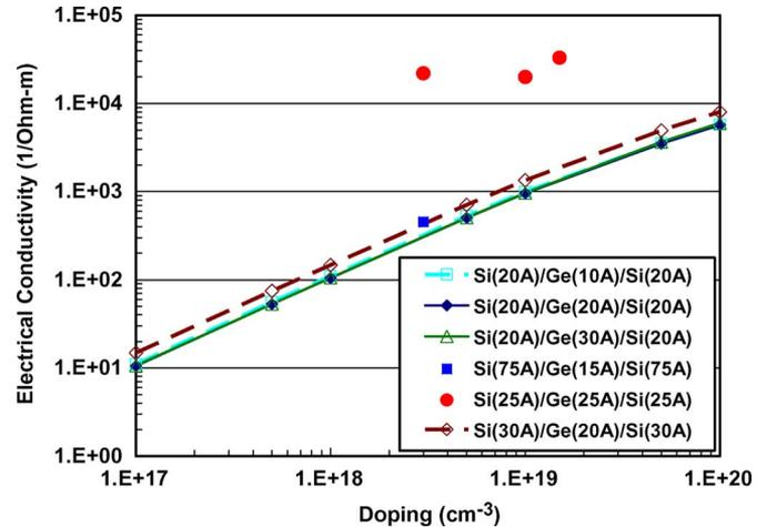
Fig. 8. Electrical conductivity versus doping for Si/Ge/Si superlattices for varying film thicknesses. Experimental data (in filled circles and square) taken from [31] and [34].
