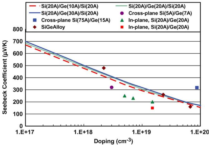
Fig. 5. Seebeck coefficient versus doping for Si/Ge/Si superlattices for various thicknesses. Experimental data taken from [8] and [30]–[33].
