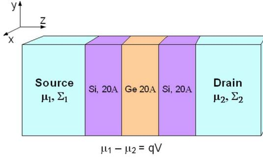
Fig. 1. Schematic representation of a Si/Ge/Si quantum-well superlattice modeled in the simulation.
