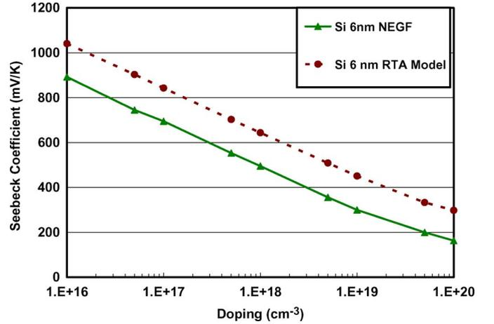
Fig. 3. Seebeck coefficient versus doping for silicon films using the NEGF and an RTA model.
