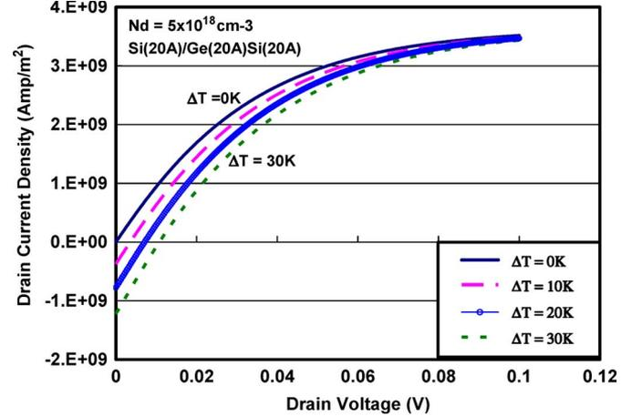
Fig. 2. Current density–voltage characteristics of a ballistic Si(20 Å)/Ge(20 Å)/Si(20 Å) quantum-well structure. Channel-temperature difference ranges from 0 to 30 K.
