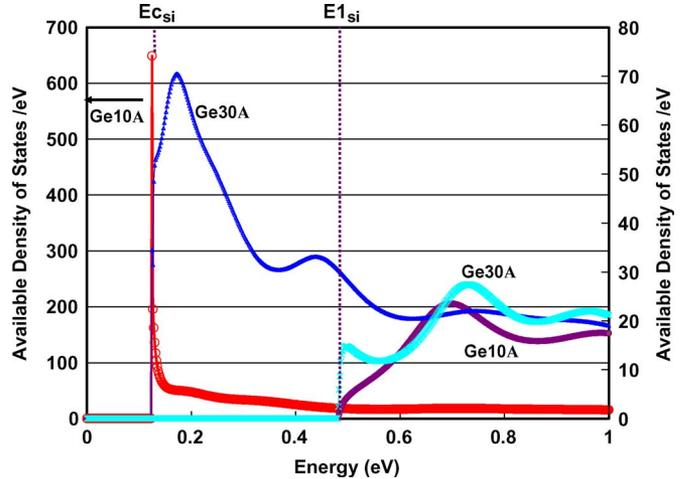
Fig. 6. Available density of states distribution versus energy for Si(20 Å)/Ge(10 Å)/Si(20 Å) and Si(20 Å)/Ge(30 Å)/Si(20 Å) superlattices.  $E_{c_{Si}}$  and  $E_{1_{Si}}$  represent the conduction band and the first subband energies in silicon, respectively. All curves are plotted against the right axis except where noted.
