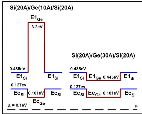
Fig. 7. Band diagram for Si(20 Å)/Ge(10 Å)/Si(20 Å) and Si(20 Å)/Ge(30 Å)/Si(20 Å) superlattices showing the conduction band and the first subband energies.
