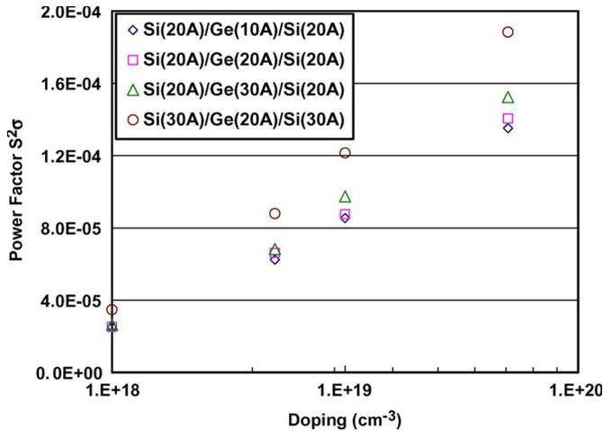
Fig. 9. Power factor versus doping for superlattices with varying film thicknesses.
