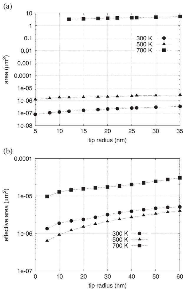
Fig. 7. Estimates of effective emission area for (a) peaked sample and (b) crowned sample.
