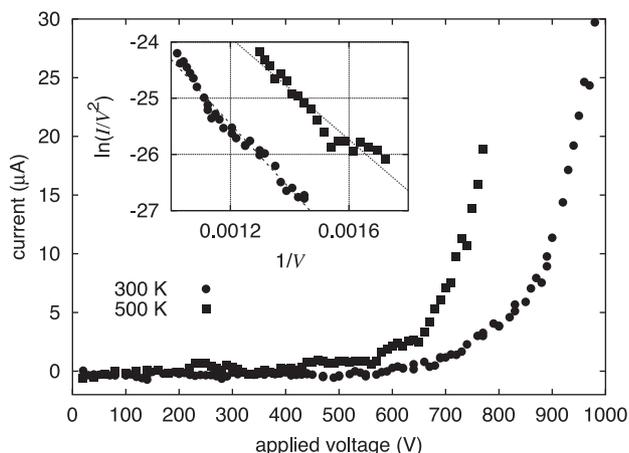
Fig. 3. Current–voltage behavior of the nanocrystalline diamond thin film.
