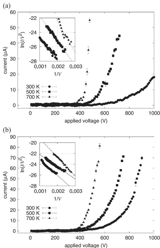
Fig. 4. Current–voltage behavior of diamond-tip emitters; (a) peaked device, (b) crowned device.
