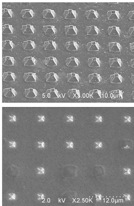
Fig. 2. Sem image of diamond tips; (a) crowned diamond microtips, (b) peaked diamond microtips.
