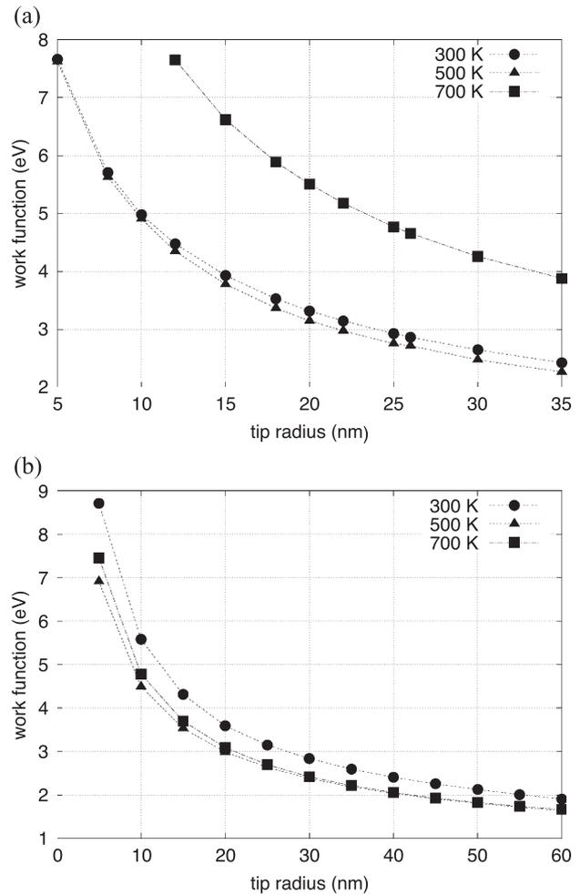
Fig. 6. Estimates of work function for (a) peaked sample and (b) crowned sample.
