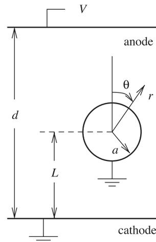
Fig. 1. Coordinates and dimension definitions used in the calculation of potentials.
