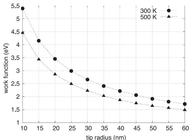
Fig. 5. Estimate of work function for nanocrystalline thin film.
