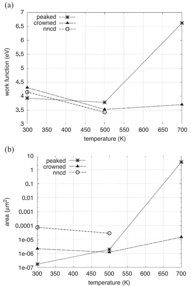
Fig. 8. Temperature dependence of (a) work function and (b) effective area.
