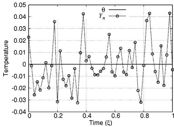
Fig. 1 The temperature response to a zero heat flux is shown with and without added noise. The normally distributed random noise has a standard deviation of  $\sigma=0.02$ . Lines are added to guide the eye.
