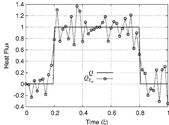
Fig. 14 The heat flux history estimates are derived from the temperatures in Fig. 12. The estimate from noisy data,  $Q_{Y_n}$ , demonstrate how small errors become amplified. The lines merely guide the eye.
