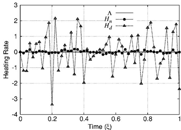
Fig. 2 The heating rate response to a zero heat flux is shown with and without added noise. The normally distributed random noise ( $H_n$ ) has a standard deviation of 0.08, and a central differencing of the noisy temperature  $Y_n$  is used to produce  $H_d$ , which has a standard deviation of 0.94. The lines connecting the points merely guide the eye.
