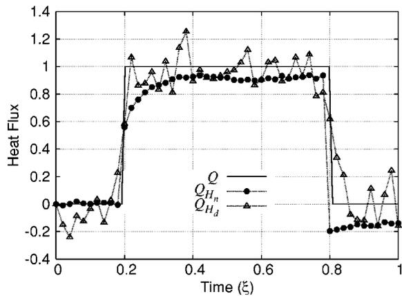
**Fig. 15** Heat flux estimates derived from heating rate data (see Fig. 13) using an exact matching scheme. Noise in the measured data is not amplified as in case of temperature data. The lines merely guide the eye.
