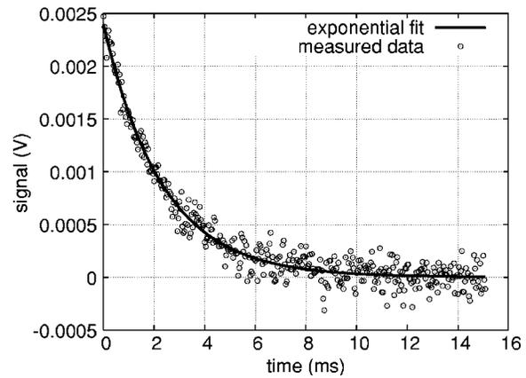
**Fig. 17** Phosphor emission from  $\text{La}_2\text{O}_2\text{S}:\text{Eu}$  after LED excitation was turned off. The data was translated so that the peak emission occurs at  $t=0$  ms. Fitting parameters are shown in Table 4.
