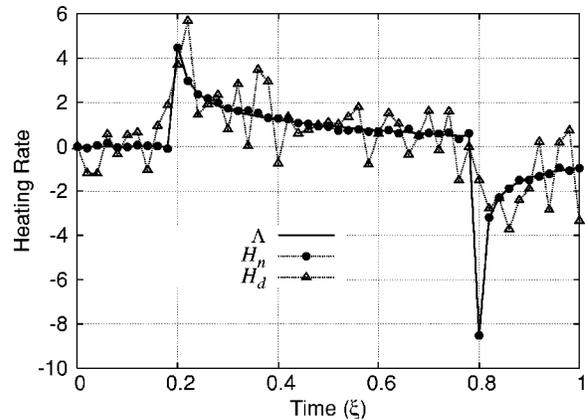
Fig. 13 Heating rate measurements of the square heat flux with and without noise
