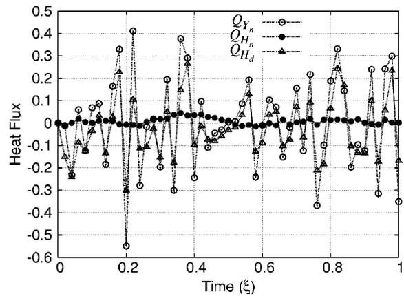
Fig. 3 The heat flux estimates of the zero flux case from temperature measurements  $Y_n$ , heat rate measurements  $H_n$  and differenced temperatures  $H_d$ . The lines connecting the estimates merely guide the eye.
