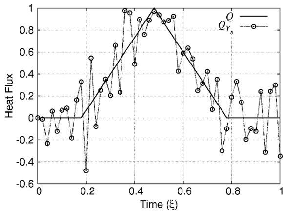
Fig. 5 The heat flux history estimates are derived from the temperatures in Fig. 4. The estimate from noisy data,  $Q_{Y_n}$ , demonstrate how small errors become amplified. The lines merely guide the eye.
